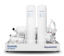
Device for the production of osmosis water through a reverse osmosis process, suitable for clinics with high water hardness. The filtering system consisting of a sediment filter and carbon filter, resin and osmotic membrane, guarantees high quality water production, suitable for supplying the autoclaves and all the practice's equipment in compliance with standard EN 13060 (<15 µs/cm).
