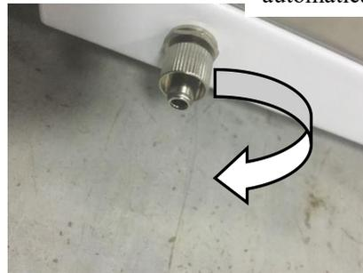
3、 After the drainage, turn the drain joint clockwise to seal the drain.
